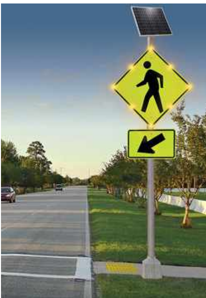
Example of a painted crosswalk with a flashing light and signage (Traffic Safety Supply Company)
