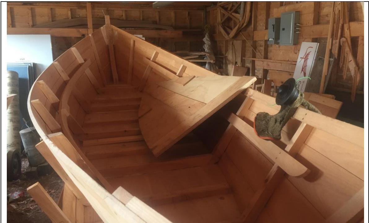
Figure 4 Interior Construction of the Nearly-Completed (Top) Dory
