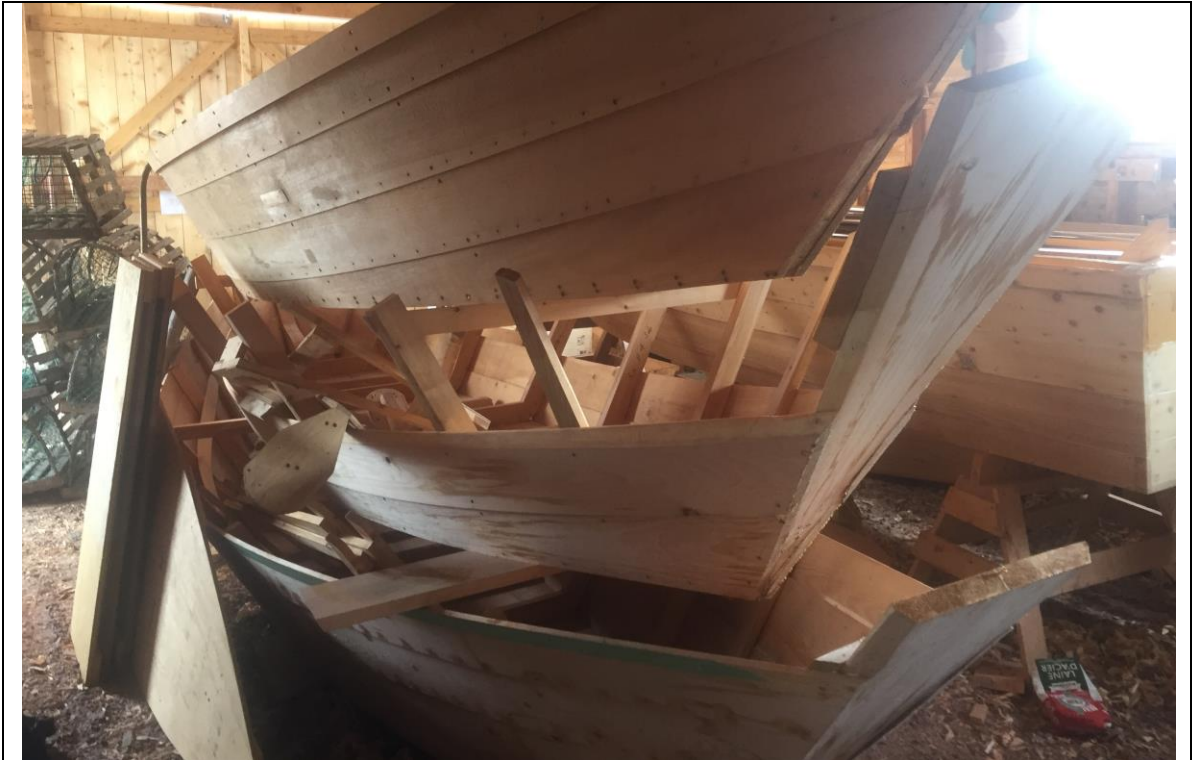
Figure 4 Interior Construction of the Nearly-Completed (Top) Dory
