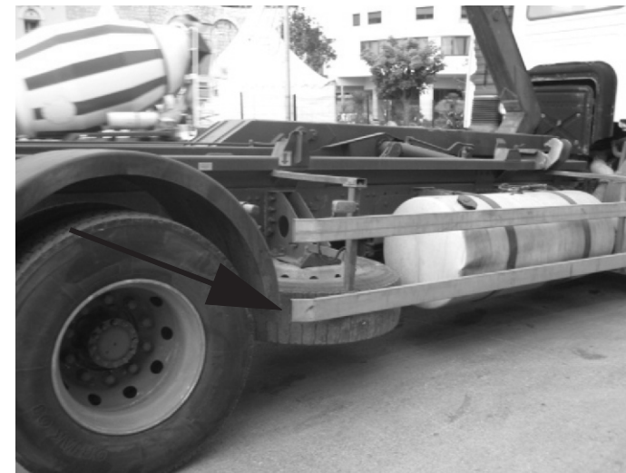
Truck-underguard (sideguard) shown protects both vulnerable road users and the trucks undercarriage
